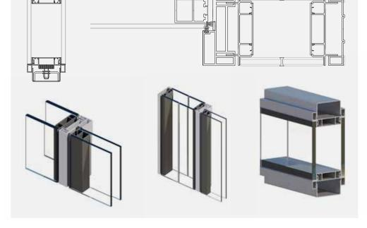
Flush frameless bonded glazing for minimal aesthetic with the benefit of high acoustic resistance. Astral frameless glazing system is both stylish and simple. It is mullion free, with minimal tracks at head, base and abutments. Astral enables a visually frameless optical with high levels of performance.
